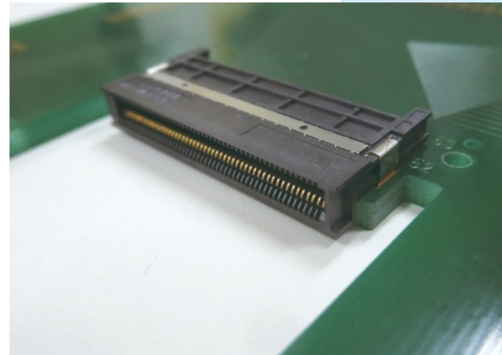
Fig.3: Host connector recessed in the PCB via mid-mount technology.
