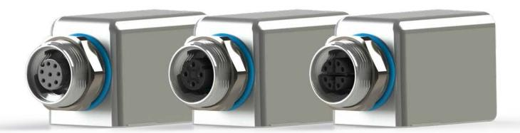
With the new switch cabinet coupler, you can easily switch from an internal RJ45 switch cabinet cabling to an external M12 cabling. Different coding variants (A8, D4 and X coding) ensure adaptation to the required transmission performance and, with the A8, offer the option of transmitting additional power.
